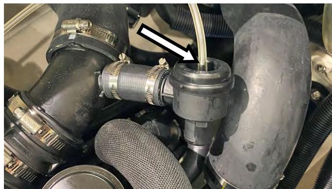
On the intake manifold, relocate forward most air intake tube cradle to runner for middle cylinder.
