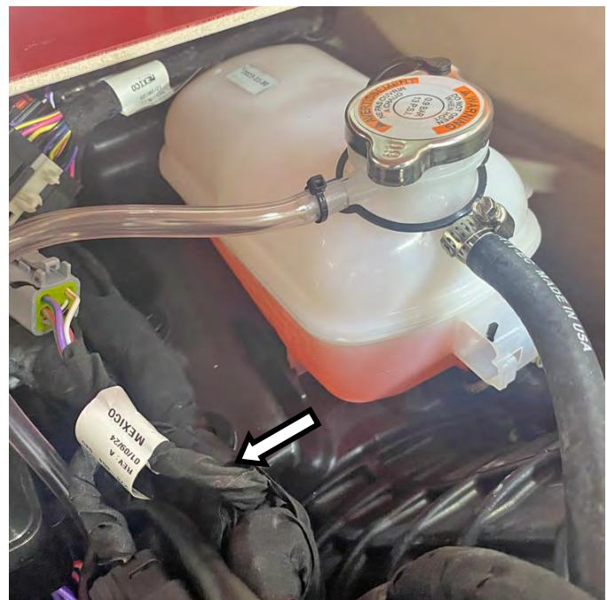
Remove coolant tank by prying locking lever away from tank and then pulling tank towards rear of craft.
