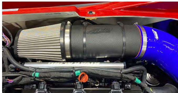
Secure Power Filter Tube to cradles on intake manifold.
