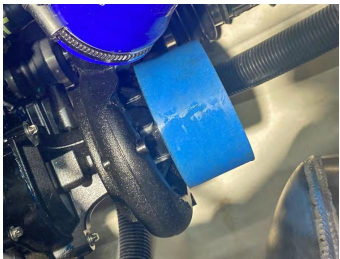
Install supplied Power Filter onto supplied Plastic Air Intake Tube and secure. **TIP: Apply glass cleaner to inside edge of Power Filter and outside edge of supplied Power Filter Tube.**
