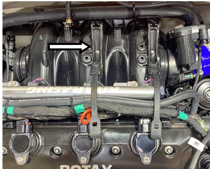
Install supplied Velocity Stack onto supercharger inlet. **TIP: Apply glass cleaner to inside of velocity stack.**
